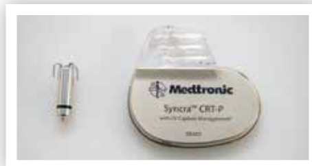
The Micra® pacemaker on the left, as compared to the size of a standard pacemaker.
